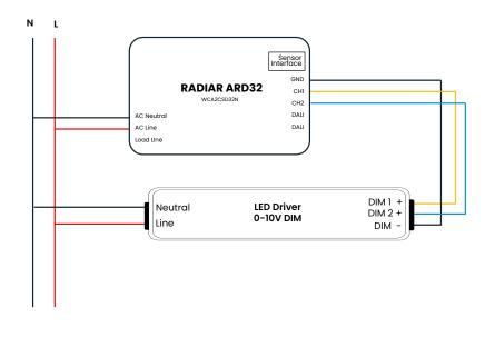
3) Connecting an external sensor with 0-3V output to the Radiar ARD32 controller using a Molex connector
